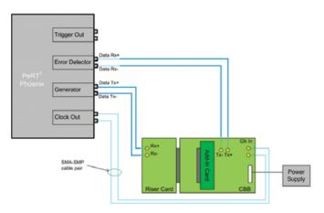
Connection diagram for Receiver Compliance Testing
