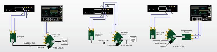
Device Transmitter Compliance Test Setup
