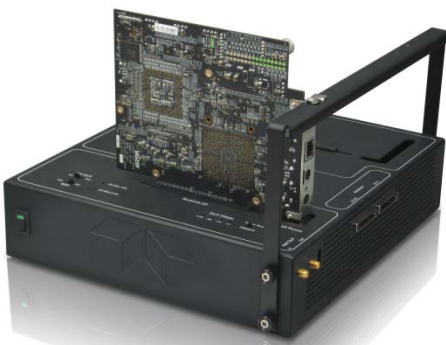
The Summit Z3-16 Exerciser acts as its own target emulator, and supports host emulation through an optional test platform.
