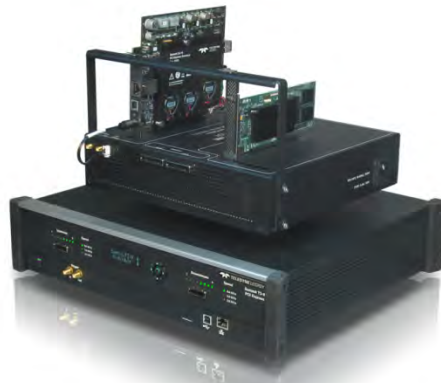
The Summit Z3-16 Exerciser, in combination with the Summit T3-8 Analyzer (shown here) or other Summit analyzers, forms the basis of standardized NVMe Conformance Test Suites developed by UNH-IOL.
