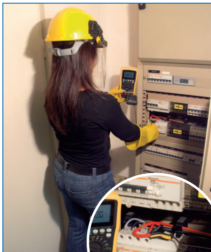
The sensors' flexibility is an advantage on industrial and domestic switchboards.
